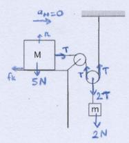
$W_{M} = 0.2 \text{ kg} \times 10 \text{ m/s}^2 = 2 \text{ N}$  $W_{M} = 0.5 \text{ kg} \times 10 \text{ m/s}^2 = 5 \text{ N}$
